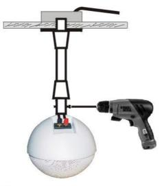
**8** Insert pole over the body stem of the Saturn speaker and add screw in with 1/4" x 20 screw.
