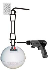
**6.** Insert pipe over the body stem of the Saturn speaker and add screw in with 1/4" x 20 screw.
