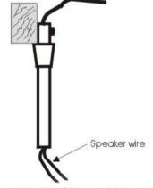
3. Run wire thru 1" pipe. Make sure you have enough to reach speaker terminal at the other end of the pipe.
