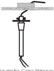
4. Run wire thru 1" pipe. Make sure you have enough to reach speaker terminal at the other end of the pipe.
