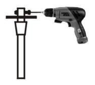
Screw in the nut and bolt into hade at the end of the pipe.
