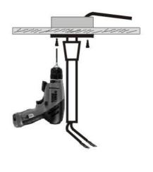
5 Screw the metal plate directly to the to the ceiling or to the gangbox.
