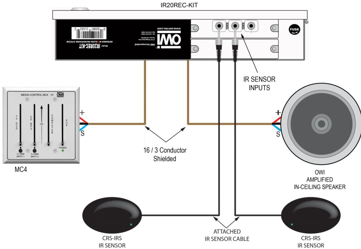
**Figure 14. Typical CRS System Connections**
