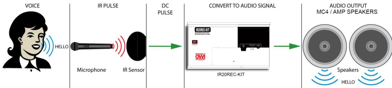
**Figure 15. IR20REC-KIT System Signal Path**
