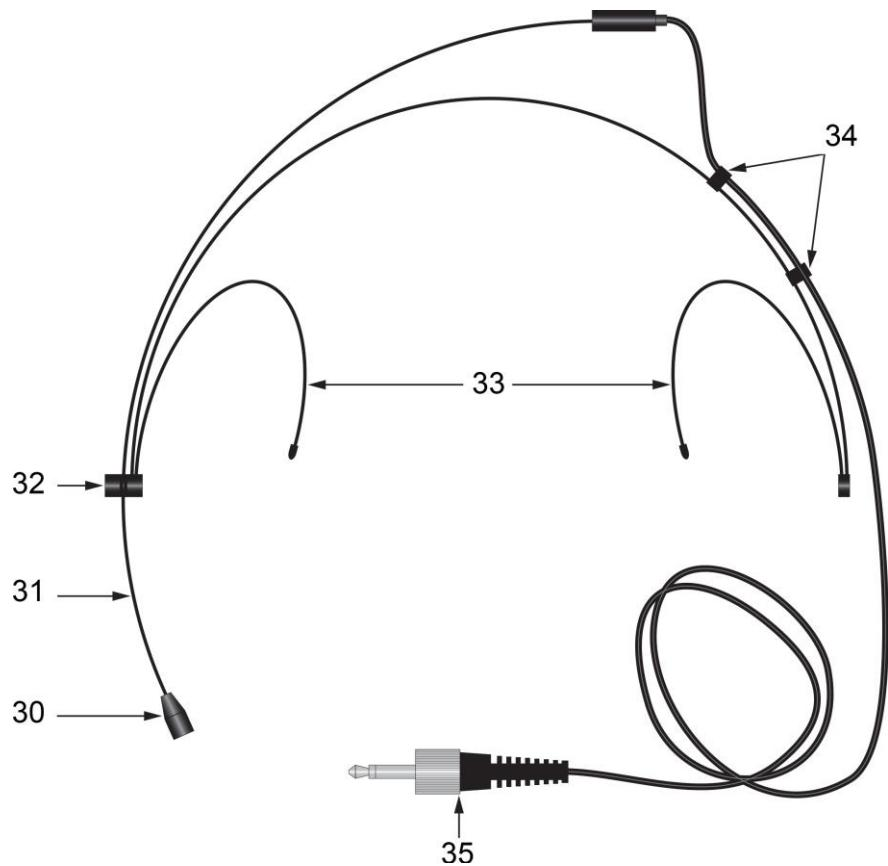
**Figure 11. CRS-HSMIC Headset Mic (Optional)**
