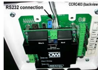
Backview of CCRC403 showing RS232 connection
