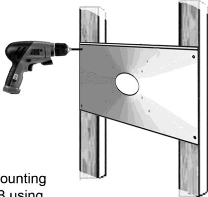
Install the mounting frame M5TB using a screw.
