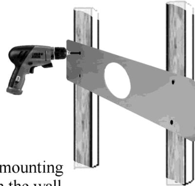
Install the mounting frame A on the wall using screw or staple.
