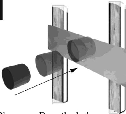
Place cup B on the hole of the mounting frame A.
