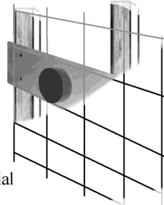
Place drywall, cement or material on front side. Do not cover cup.
