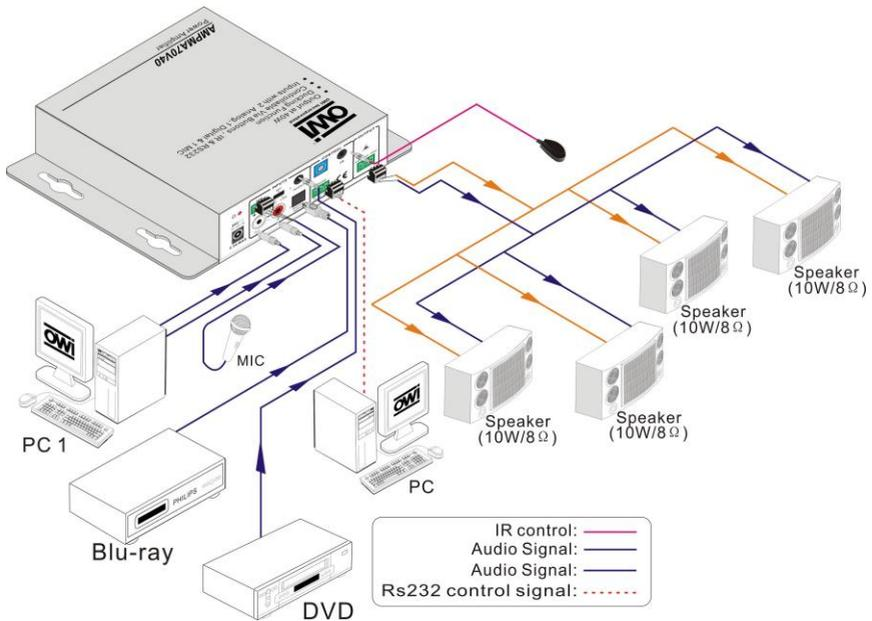
Figure 3 System Diagram
