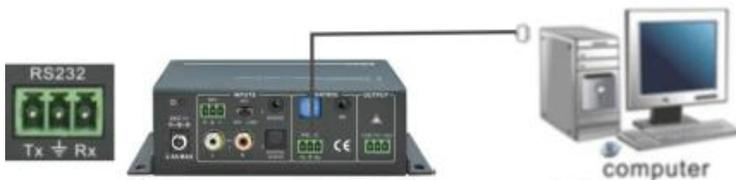
Figure 10 Connection of RS232 Port
