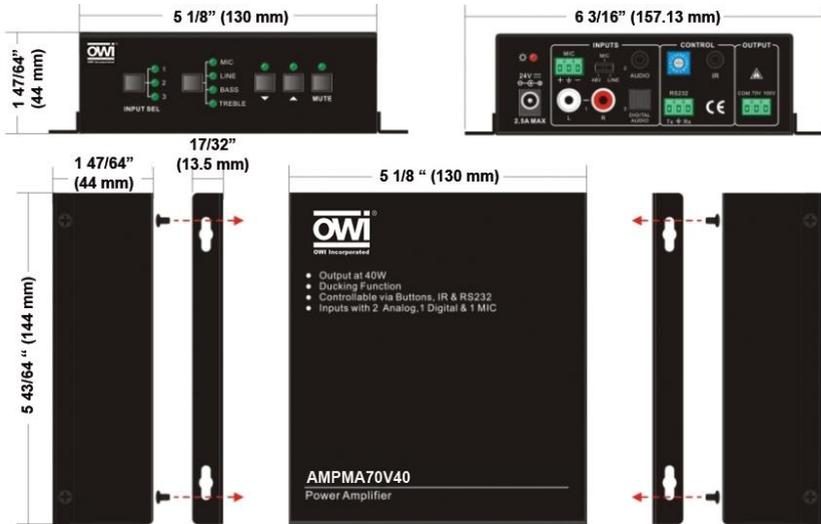
Figure 13 Panel Drawing
