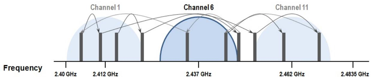
Figure 3: FHSS and DSSS transmissions will collide when the FHSS transmitted hops to a portion of the operating band occupied by the DSSS transmitter.
