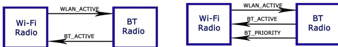
*Figure 4: With two-wire coexistence (left), the radios are aware of the transmit status of the coexistent radio and can thereby refrain from transmitting simultaneously. Three-wire coexistence (right) adds an indication of the priority of the Bluetooth transmission.*
