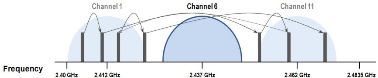
*Figure 5: With AFH, FHSS devices avoid DSSS channels to allow for improved performance for both Bluetooth and Wi-Fi devices.*
