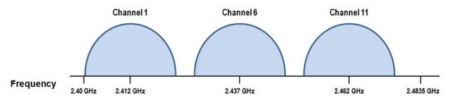
Figure 2: With Direct Sequence Spread Spectrum, the signal is transmitted on a continual basis across a range of frequencies referred to as a channel.
