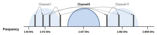
Figure 5: With AFH, FHSS devices avoid DSSS channels to allow for improved performance for both Bluetooth and Wi-Fi devices.
